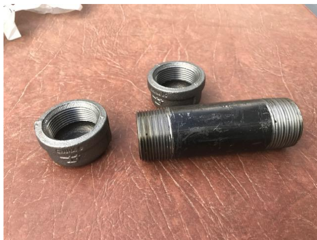
Figure 1 "Crucible": a 1 1/4" pipe fitting with two end caps.
