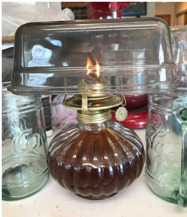
Figure 3 A heat resistant glass dish over a linseed oil lamp for making lamp black pigment.
